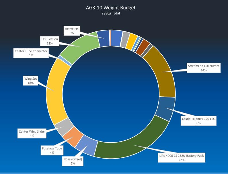
43% Propulsion and Energy Storage46% Structural Components11% Controls and Sensor Package
